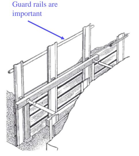
The struts between the sides of the trench are metal 'trench struts', which are adjustable so that they can be firmly braced against the supports. Timber struts, tightened by the use of wedges at the ends, are just as effective.
