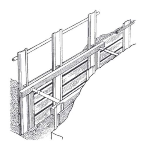
An example of how a larger excavation can be supported and provided with safety barriers
